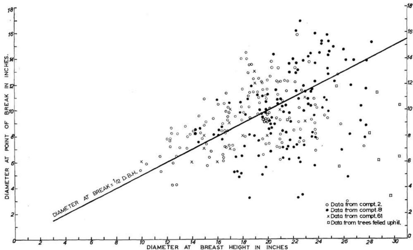
FIG. 1: Diameter of *P. radiata* stems at point of break in clearfelling operations on 25° slopes at Golden Downs, plotted against d.b.h. (December, 1965).
