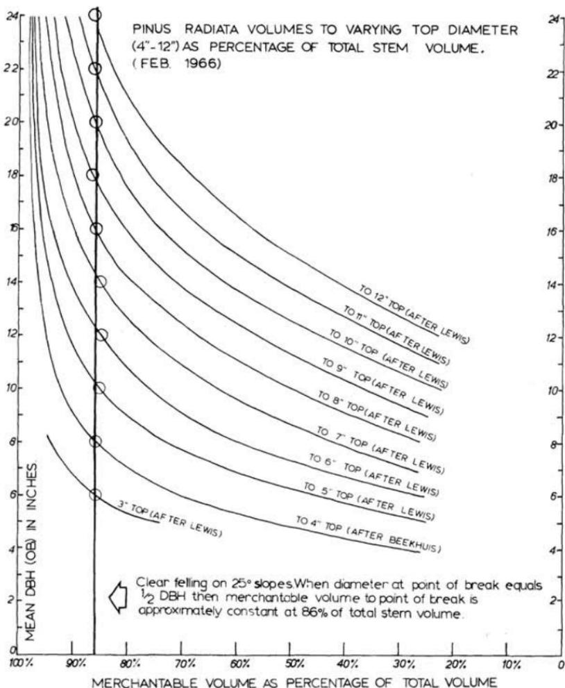
FIG. 2: Merchantable volume, below point of stem breaking, as a percentage of total stem volume for trees of given d.b.h.o.b.
