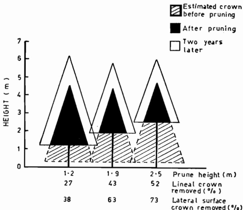
FIG. 1: Crown profiles for three pruning levels (sub-plot treatment).
