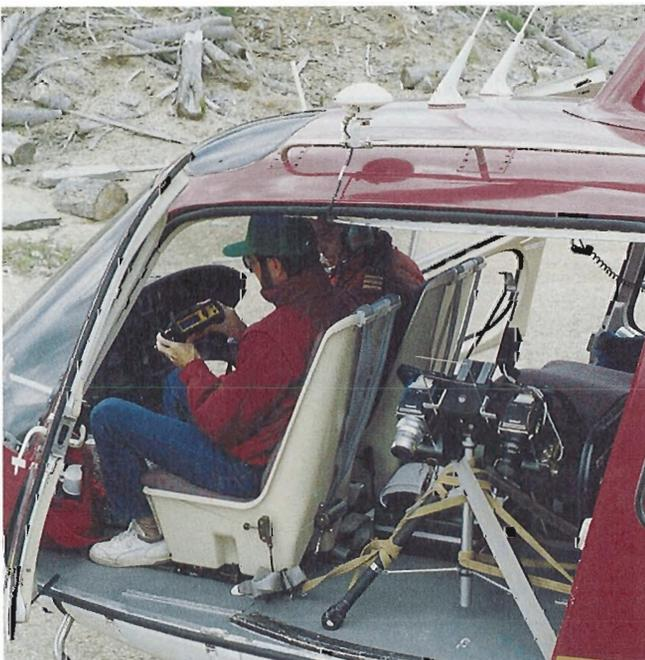
Figure 2. Using a GPS unit as a navigation aid for low-altitude aerial photography.
