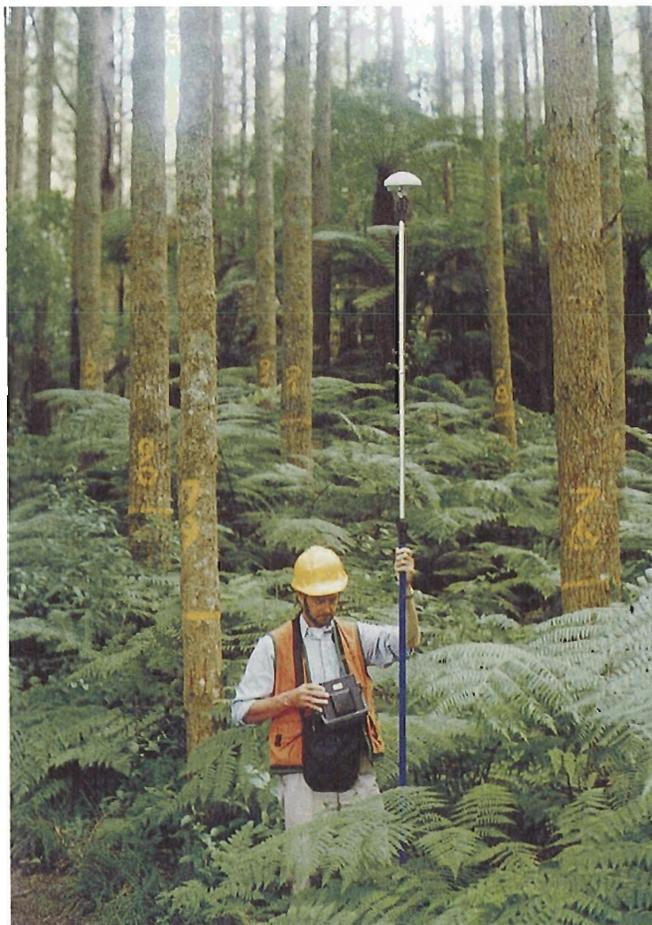
Figure 1. Evaluating a GPS unit to record the location of a sample plot in a forest stand.
