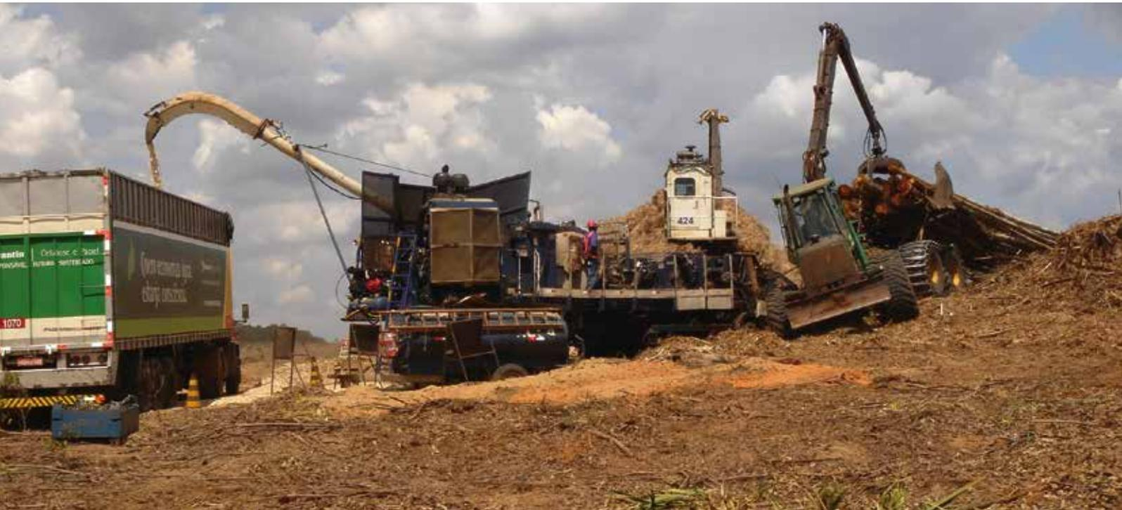
Full tree harvesting with integrated grapple skidder extraction, on-site chipper and chip liner trucking, VCP Company, Sao Paulo, Brazil
