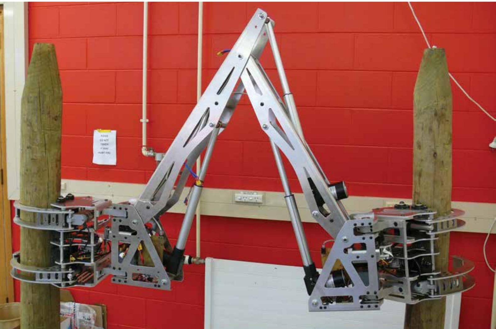
Tree-to-tree locomotion robot – Stick Insect conceived by Scion and built by Department of Mechanical Engineering, University of Canterbury
