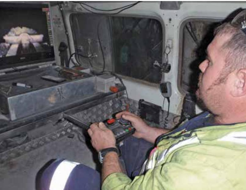
Teleoperation of a LHD machine in a New Zealand underground mine. The operator is viewing a video monitor showing the scene in front of the machine
