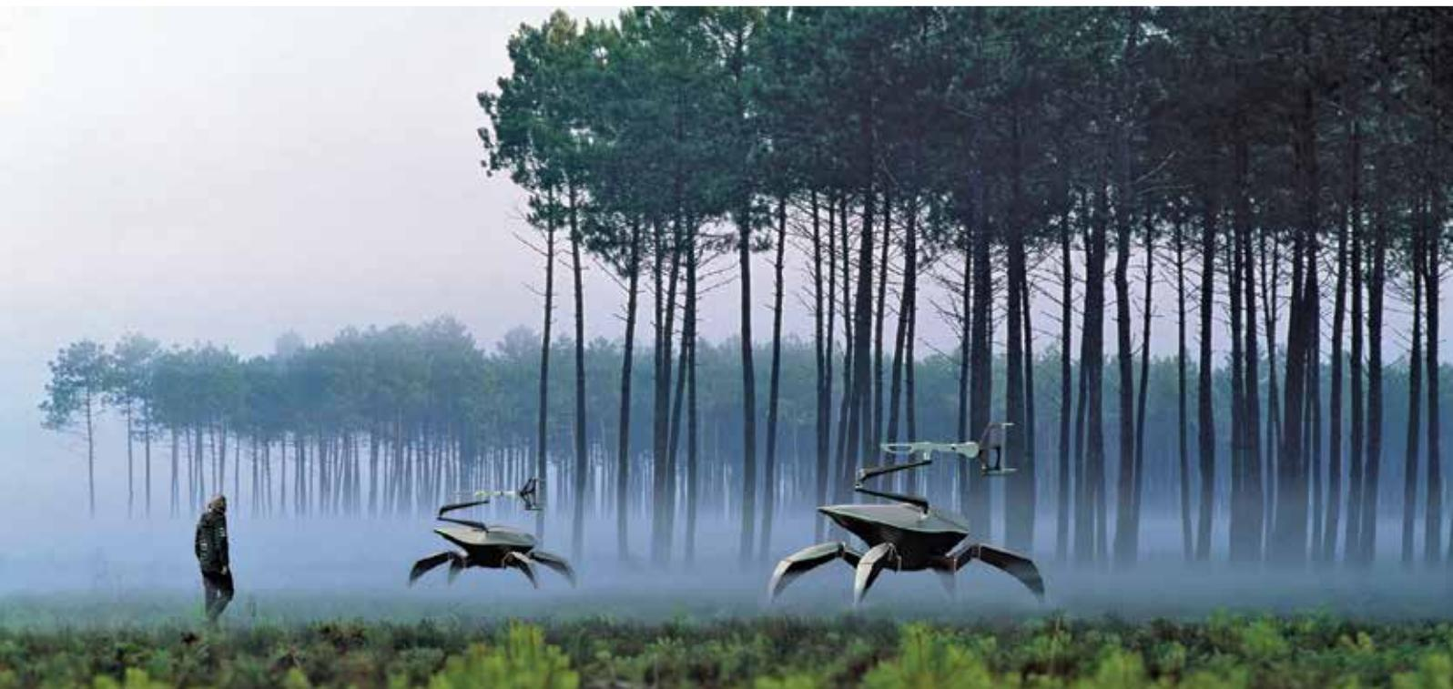
Autonomous harvester concept machine developed by design students in Sweden. (Photo: Ludwig Östman, Skogstekniska klustret)
