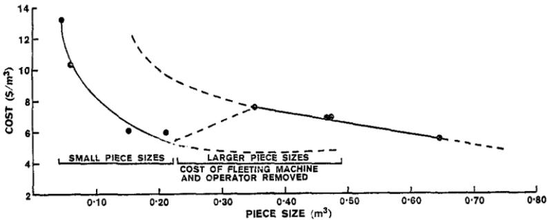
FIG. 2: Production thinning — radiata pine. Ground extraction-cost trend/ $m^3$  on landing 1977, with and without fleeting machine and operator.
