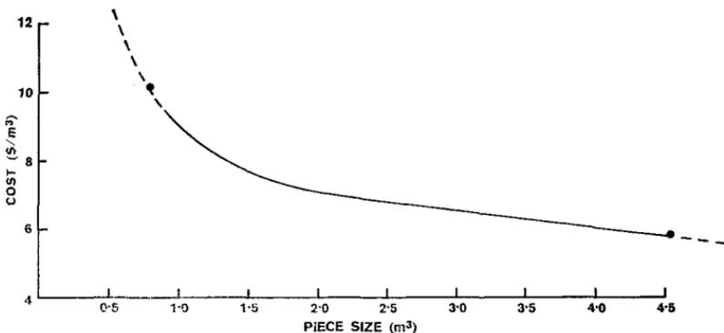
FIG. 8: Clearfelling — radiata pine. Cable system-cost trend/m<sup>3</sup> on landing 1977.
