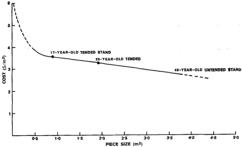
FIG. 4: Clearfelling — *radiata pine*. Ground extraction-cost trend/ $m^3$  on truck 1977.
