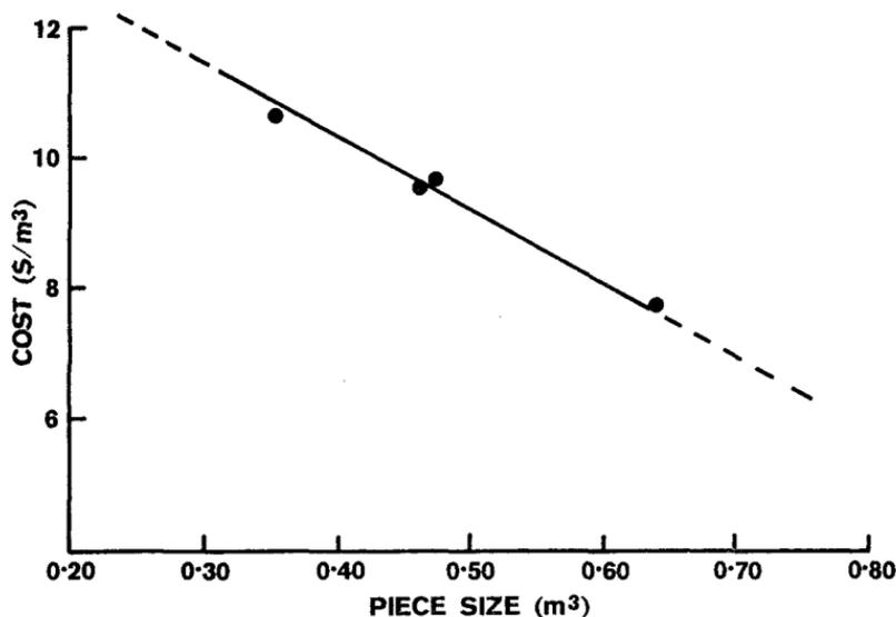
FIG. 6: *Production thinning — radiata pine. Cable system-cost trend/m<sup>3</sup> on landing 1977.*
