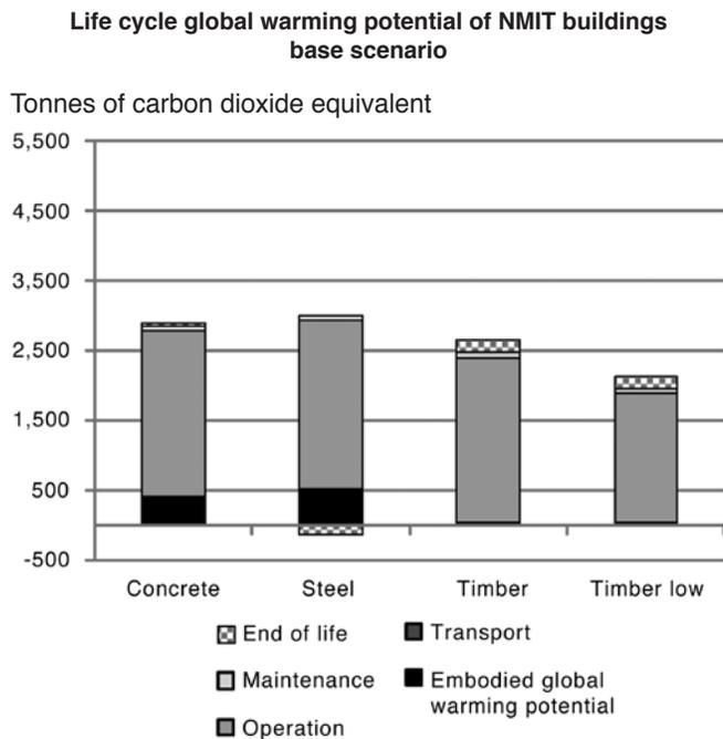
Figure 5a: Global warming potential for each building, by life cycle stage, for whole life cycle including operational energy – current end-of-life scenario
